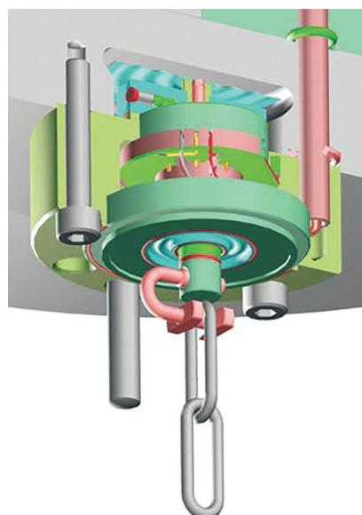
Carefully place transmitter and displacer onto the container flange **140**. Make sure the seal is accurately positioned. **Avoid impacts and jolting under all circumstances**. Tighten studs **142** and nuts **143**. Apply recommended torque (see tables below).
