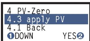
→ With YES ② the current process value (Level: Displacer not in the medium) is taken over as the physical zero point.
