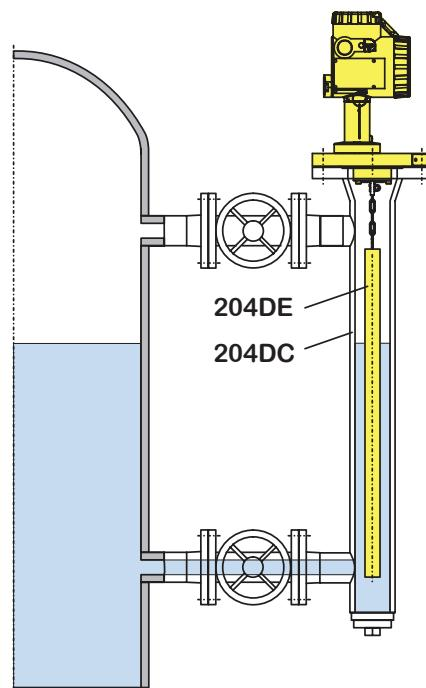
Transmitter and Shut-off device
