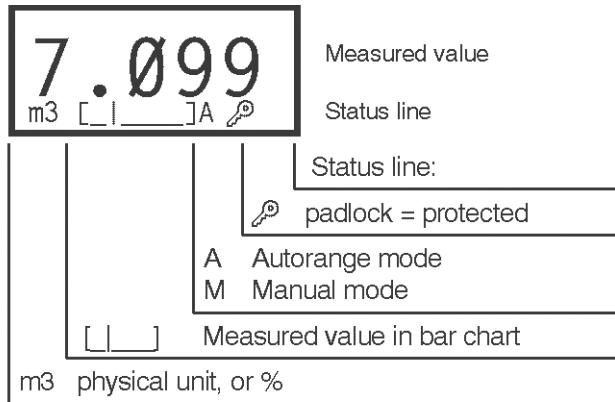
The operational view is the display in normal operation.
