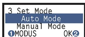
With ① MODE you switch from Autorange- to Manual Mode. If this is to expect a change in the output value, a message appears. After confirming with OK ② back to the main menu.
