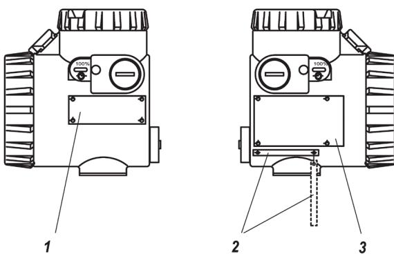
The transmitter is identified with three labels. The transmitter nameplate 3.1 shows the Model Code of the transmitter, which clearly describes the device. The certificate data and the serial No. are entered on the amplifier nameplate 3.3. The TAG No. label 3.2 with the Tag No. is located underneath (optional). Data about the permissible static pressure and the displacer are documented on the data label 3.4 on the process connection flange.
