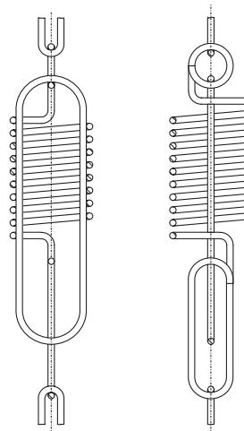
It is hooked onto the suspension chain of the displacer in place of 7 chain links (105 mm). This spring is specially matched to the resonance frequency of the displacer and is made of stainless steel (material 1.4310, max. operating temperature 250°C).
