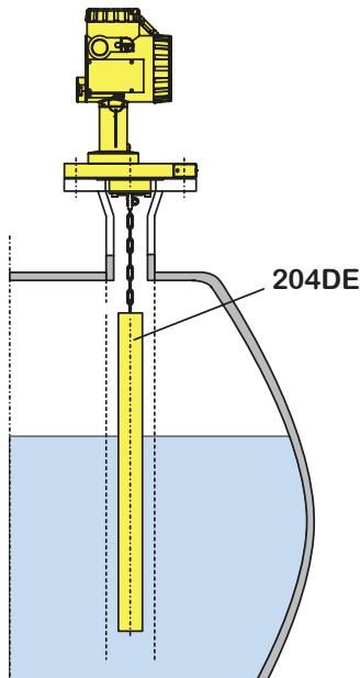
Transmitter at Connection flange Displacer 204DE in protection cage/tube
