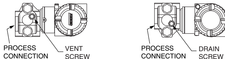
Figure 16. Horizontal Mounting - Cavity Venting and Draining
