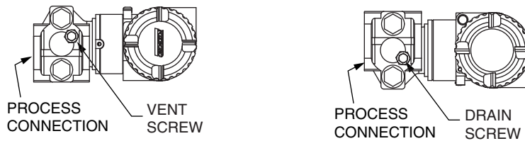
Figure 16. Horizontal Mounting - Cavity Venting and Draining
