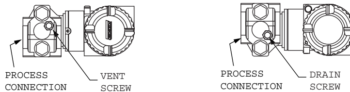
Figure 16. Horizontal Mounting - Cavity Venting and Draining
