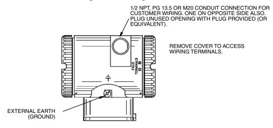
Figure 14. Identification of Field Terminals
