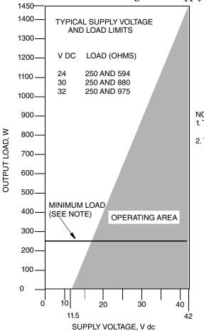
Figure 15. Supply Voltage and Loop Load
