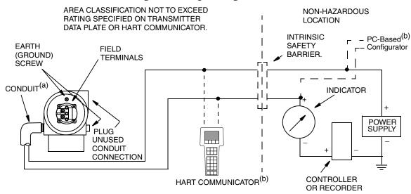
Figure 16. Loop Wiring Transmitters
