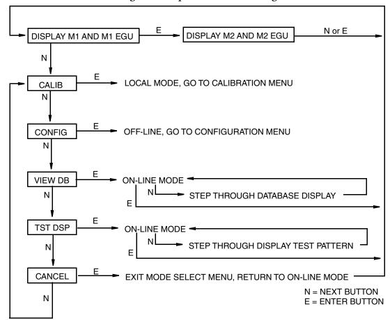
Figure 20. Top Level Structure Diagram
