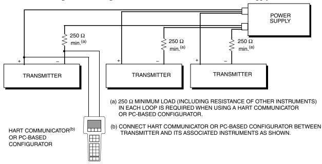
Figure 17. Wiring Several Transmitters to a Common Power Supply
