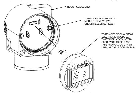
Figure 30. Replacing the Electronics Module Assembly and Display
