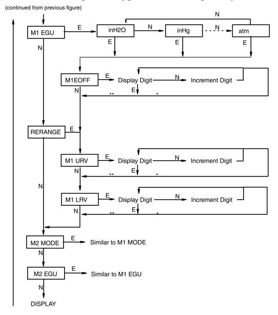
Figure 28. Configuration Structure Diagram (2 of 3)
