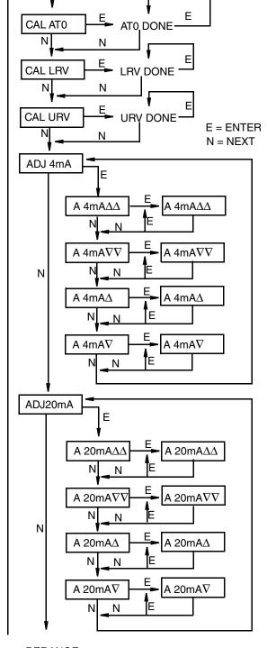
Figure 25. Calibration Structure Diagram (1 of 2)
