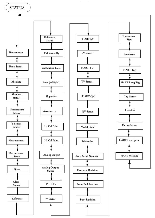
Figure 23. Status Mode Structure Diagram for 876PH-T Transmitter
