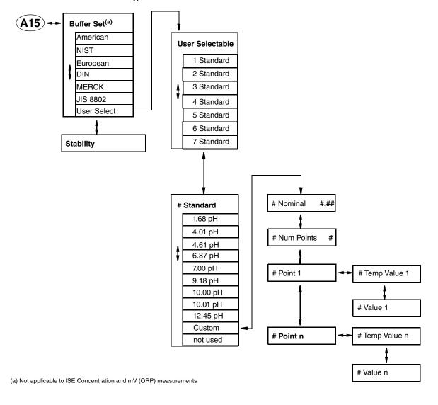
Figure 73. Calibration Parameters Structure
