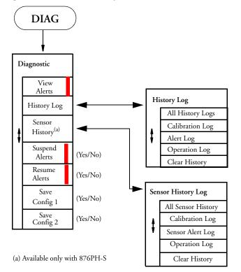
Figure 31. Diagnostic Mode Structure for 876PH-T and 876PH-S Transmitter
