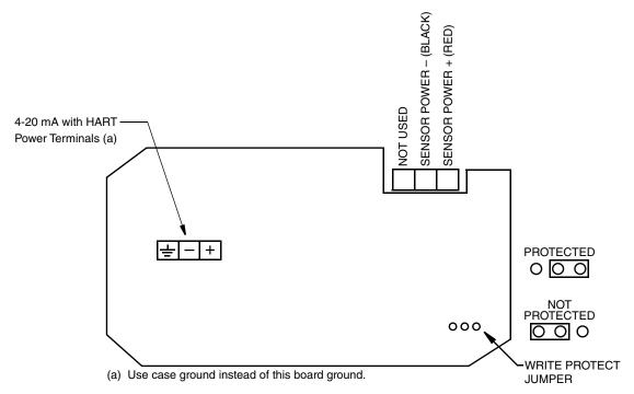
Figure 2. Wiring Connections for 876PH-S Transmitter
