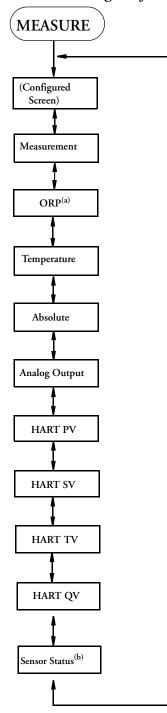
Figure 22. Measure Mode Structure Diagram for 876PH-T and 876PH-S Transmitter
