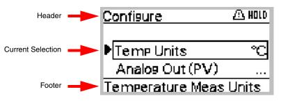
Figure 17. Three Lines That Can Be Scrolled if Text Is Too Long to Display
