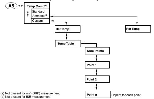
Figure 63. Temperature Compensation Structure
