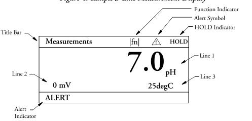
Figure 4. Sample 3-Line Measurement Display
