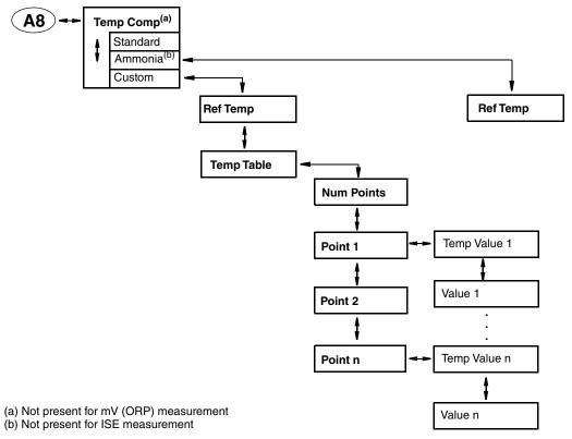
Figure 46. Measurement Display Format Structure
