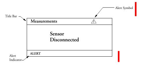
If the alert is related to the sensor, then the Alert icon in the Di agnostics menu displays: User Alert, Sensor Missing.
