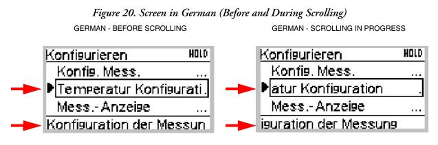
Auto Scroll stops immediately when you make a selection using any of the controls.
