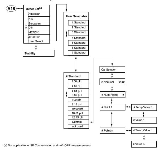
Figure 55. Calibration Parameters Structure
