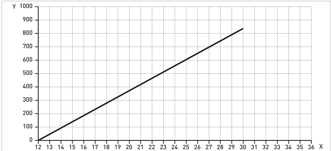
Figure 8-4: Minimum power supply voltage for an output of 21.5 mA at the terminals (Non-Ex and Hazardous Location approval (Ex i / IS))
