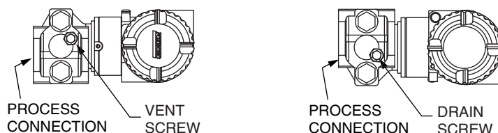
Figure 21. Horizontal Mounting - Cavity Venting and Draining
